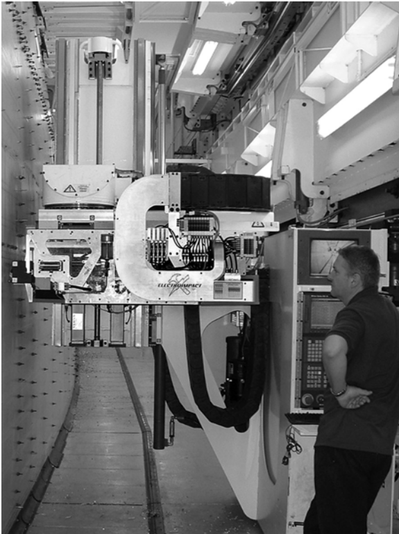
Figure 4. Y-Shift in the Raised Position
